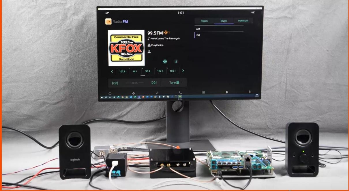
During the live session, a demo is shown in which the ADP board is running an Android Broadcast Radio App using both the NXP and Skyworks based USB Tuner available with Radio Tuner SDK interchangeably. This text replaces the demo in the PDF version for technical reasons.
